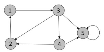
Note that each vertex (line) has an arrow that points in a specific direction; that is what makes the graph a directed graph. Note edge (node) number 5 which has an arrow that points to itself; that is a cycle. Cycles like that can cause issues such as causing an infinite loop. Those sorts of issues can be solved by using a directed acyclic graph that does not allow such cycles which we will cover next.
