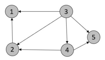
Note again that each vertex has an arrow which specifies a direction and that there are no cycles making this a directed acyclic graph. Note that there is not one specific edge (node) that can be considered the root of the graph.
