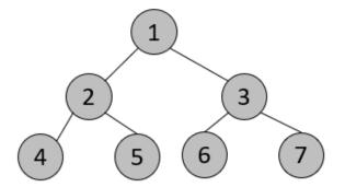
Notice the root, node number 1 and that ever other node that appears is unique. Notice also that there is no direction associated with the lines that appear between the nodes.
